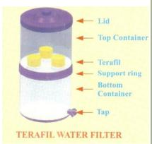
The Terafil Water Filter is an assembly of six parts:
